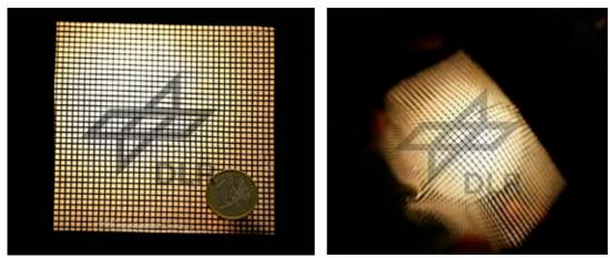
Figure 6: left: DLR tactile sensor; right: wrapped around a light bulb
