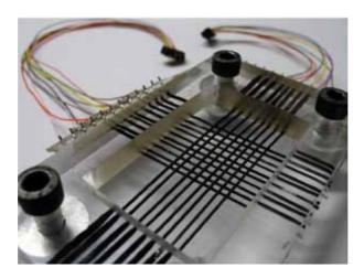
Figure 5: Prototype of the coated wire sensor
