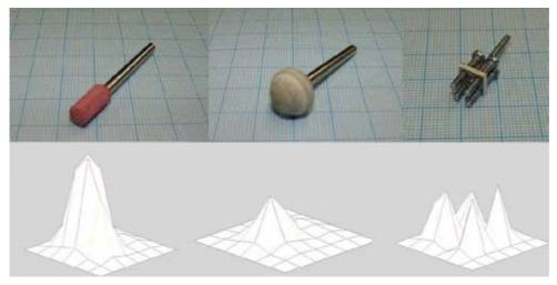
Figure 3: Indenting the DLR tactile sensor. The below graphs shows the measured voltages when indented with the above probes.
