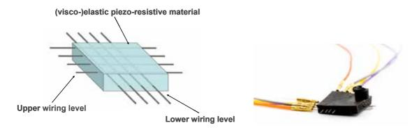
Figure 1: First Generation DLR touch sensor
