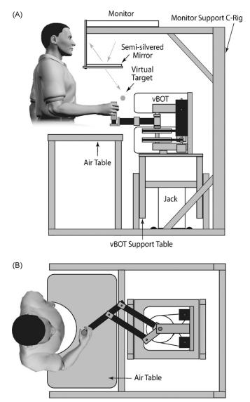
**Fig. 4.** The vBOT virtual reality system. (A) Side view showing the vBOT, its adjustable-height support table and the C-Rig which supports the monitor and semi-silvered mirror. The C-Rig is designed to provide a large unobstructed workspace. The vBOT table incorporates a jack for height adjustment. (B) Plan view showing location of air table.
