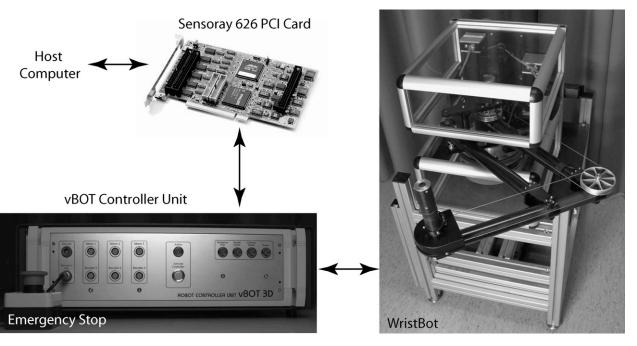
Fig. 1. The components of a vBOT system, showing the vBOT manipulandum, controller unit, emergency stop, and interface card.
