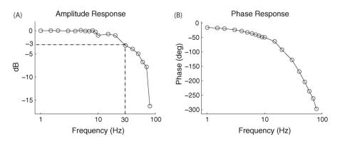
Fig. 7. Frequency response of the StiffBOT. (A) Amplitude plot showing that the response falls to -3 dB at a frequency of 30 Hz. (B) Phase plot.
