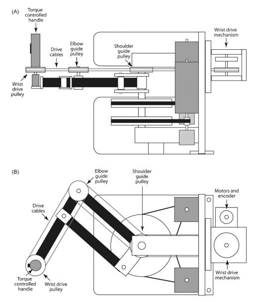
Fig. 3. Anatomy of the WristBOT, showing additional cable drive mechanism. (A) Side view showing the cable routed from the handle, via the guide pulleys, to the drive mechanism mounted on the base plate. (B) Top view.
