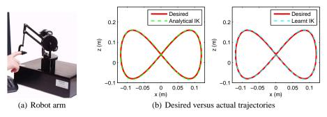
Figure 5: Desired versus actual trajectories for SensAble Phantom robot arm
