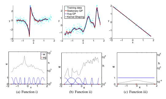
Figure 3: Predicted outputs using a stationary GP, our augmented nonstationary GP and local kernel shaping. Figures on the bottom show the bandwidths learnt by local kernel shaping and the corresponding weighting kernels (in dotted black lines) for input query points (shown in red circles).
