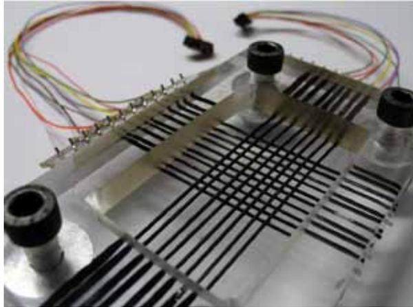
**Figure 5: Prototype of the coated wire sensor**
