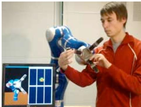
**Figure 9: UEDIN setup of tactile sensors mounted on Schunk dexterous hand SDH-2 for tactile discrimination.**
